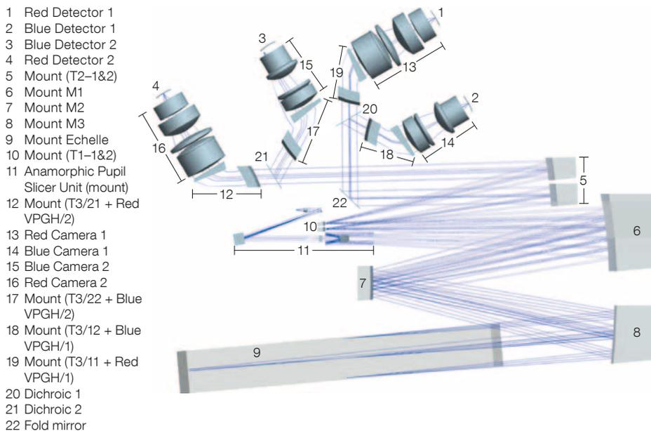
entrance. In the spectrograph the pupil is made highly anamorphic and sliced into six parts, which pass through the 1.7-metre long echelle and the collimating system of the spectrograph, after which they are divided into two separate paths (Blue and Red). Each path is imaged onto two cameras, each equipped with  $9 \times 9 \text{ cm}$  CCDs. Figure 3 shows the optomechanical concept. The cross-dispersed format enables the whole range, 380–710 nm, to be
